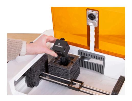
10. Next, you'll place the laser head on the magnetic dock — it's the black square mounted on top of the two silver laser rails. Set the laser head on the dock with the laser ribbon cable at the back and the Glowforge logo reading left to right. You'll feel it magnetically snap into place.
