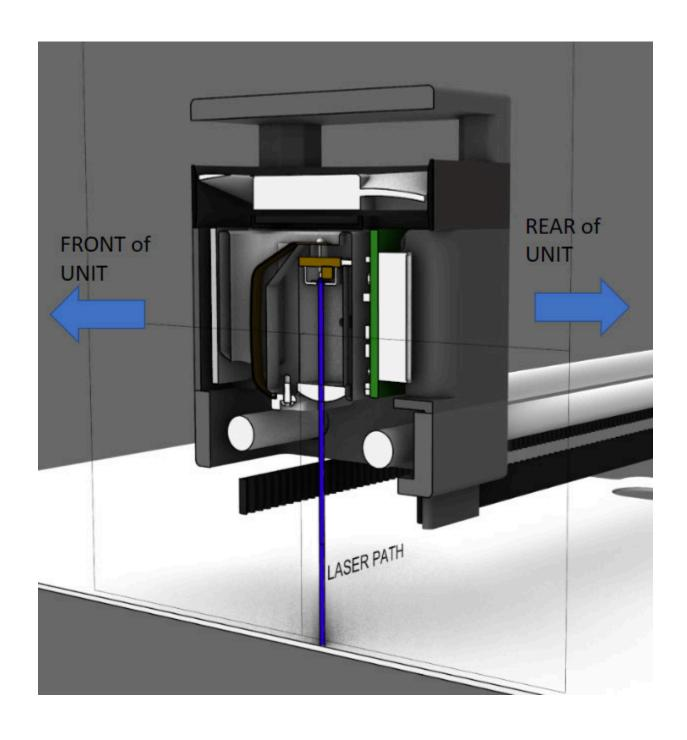
Figure 2: Laser Beam path as viewed from inside the safety enclosure.
