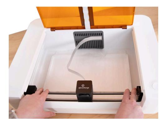
14. Now, still holding on to the end caps, gently push the laser arm all the way to the rear of the printer. Again, apply some pressure to make sure both end caps are flush with the rear.
