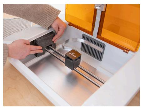
6. Lift the laser head, separating it from the magnetic dock. Slide the laser head into its foam piece with the logo facing up. The laser ribbon cable
