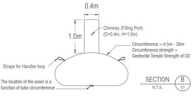
N.B. ProTube may be constructed to a variety of sizes in both length and diameter. Please speak to Global Synthetics for your specific project requirements.
