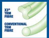
X3° 3-dimensional fibres are incorporated into all Propex erosion control products to create a thick matrix of voids to trap and house more sediment, soil and water to promote rapid vegetation growth. Superior
