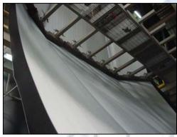
Picture (3) shows the White/Black being produced by blown film extrusion.
