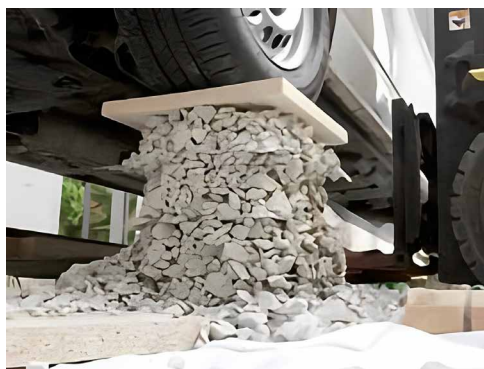
Fig. 5 Interlocking effect of Secugrid®/Combigrd®. Radial movements on the base course causes a torsional momentum in the junctions.
