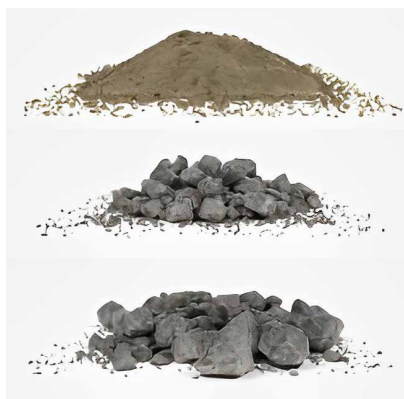
Fig. 7 Aggregate used over the geogrids during installation damage testing (from top to bottom): 61 (0 - 5mm) 62 (0 - 32mm) 63 (0 - 75mm)
