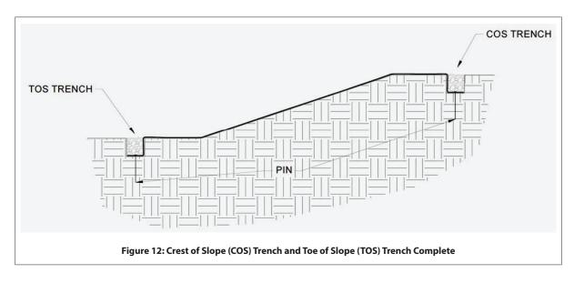
8. Backfill and compact the TOS trench. (Figure 12)
