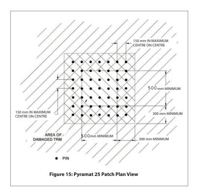
4. Install pins at 150 mm (max) centres. For larger areas of damage, pins should be installed to match existing pin pattern. Once Pyramat® 25 is in place, vegetate per project specifications.
