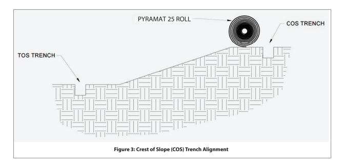
3. Secure Pyramat® 25 with pins in the COS trench. Pins should be made of mild steel with a 4 mm minimum diameter, and a length between 150 and 300 mm with sufficient ground penetration to resist pullout (Figure 4). Longer pins may be required for looser soils. Heaver metal stakes may be required in rocky soils. Suggested placement of pins for the COS trench is along the bottom of the trench with pins on 300 mm centres. Pins should also be installed on panel edge overlaps in the COS trench.
