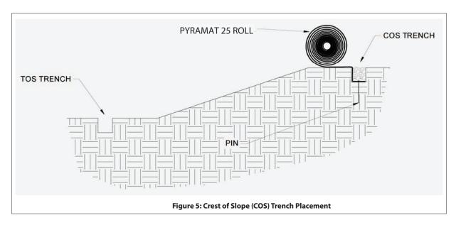
5. Unroll the Pyramat® 25 roll on the slope surface in the area to be armoured (Figure 6). Ensure that Pyramat® 25 has intimate contact with the ground and all irregular surfaces beneath Pyramat® 25 are removed.
