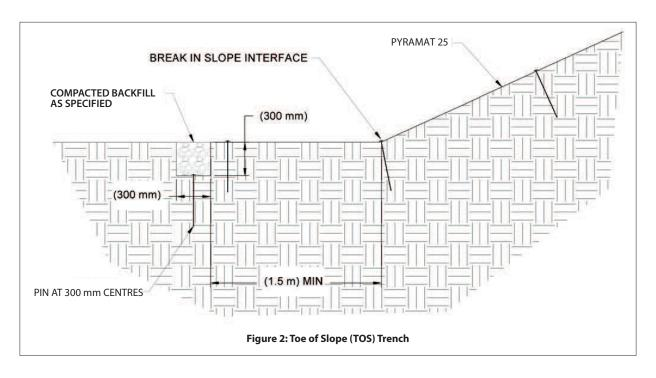
Pyramat® 25 Turf Reinforcement Mat- Slope Installation and Maintenance Guidelines
