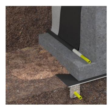
The HDPE cuspated core of the geocomposite provides a free flowing drainage void. The cusps are designed to support the geotextile which is bonded to the core, to ensure that it doesn't deform into the drainage void under the pressure of the backfill material. Deckdrain is designed to allow flow in all directions, unlike linear or pipe systems.
