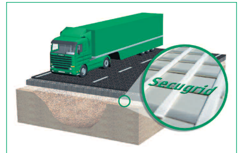
Figure 4 Secugrid® reinforcement over areas prone to subsidence
