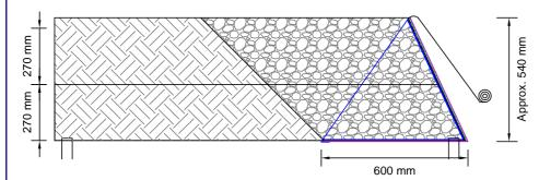
**Step 7** - Continue placing reinforced fill in 270mm lifts and compact as described in steps 5 & 6 until the complete Terralink unit is backfilled.
