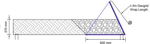
**Step 6** - A coarse rock between 75 to 200mm in diameter shall be carefully placed 600mm behind the Terralink panel avoiding damage to the Terralink struts. The rock is brought up to the height of the compacted reinforced fill as shown. Should shotcrete be omitted and Landlok 450 be installed, a suitable vegetative soil shall be placed within the rock voids to assist with vegetation growth. Vegetation to be established and nurtured through hydroseeding techniques by others.
