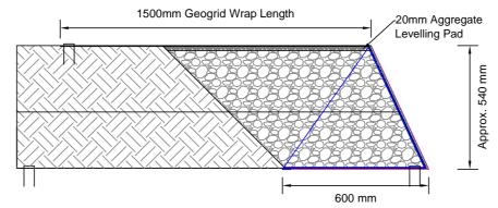
**Step 8** - Place 20mm Aggregate Over Rock To Create Level Platform For Next Terralink Panel. Fold back the erosion control blanket (if installed) and 1.5m of ACEgrid.on top of the compacted reinfoced fill. Pull the geogrid taught and install u shaped steel pins to prevent movement of geogrid while placing next Terralink welded mesh unit.
