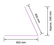
Step 1 - Once the foundation has cut to it's final level and compacted to meet the required bearing capacity, place the Terralink welded mesh facing on the level foundation. The Terralink panels are 2.4m long by 0.54m high(with a approximate tolerance of 3%) and is folded to a set facing angle of 65 degrees. Adjacent Terralink panels shall be overlapped by one mesh opening or a minimum 50mm. Alternatively the adjacent panels may be butted together and securely laced using hog rings.
