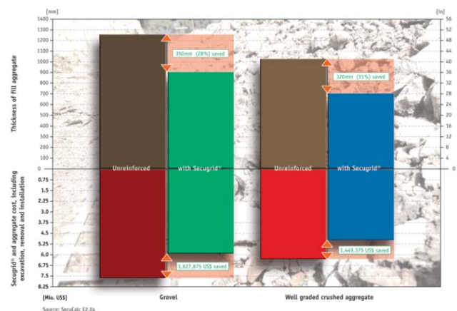
Fig. 15 Aggregate thickness and cost savings for unreinforced and Combigrid® reinforced unpaved roads
