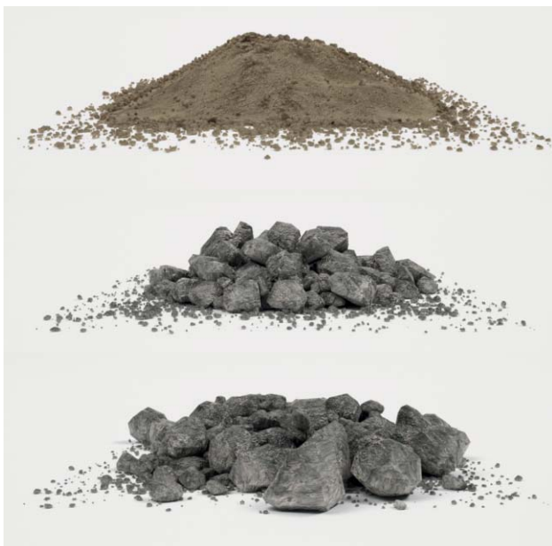
Fig. 7 Aggregate used over the geogrids during installation damage testing (from top to bottom): G1 (0 - 5mm) G2 (0 - 32mm) G3 (0 - 75mm)
