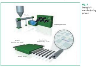
stretch the ribs and orientate the polymers into high tenacity flat bars (figure 4). These ribs are fed into the welding equipment where cross machine direction ribs
