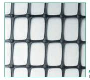
the sheet in both directions, orienting the polymers, developing tensile strength. However, there is a little orientation in the junction.
