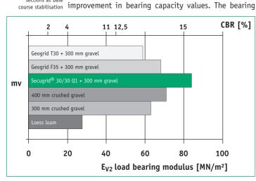
capacity results ( $E_{V2}$ ) with Secugrid<sup>®</sup>, averaged at 95.2 MN/m<sup>2</sup> (CBR: 14.5 - 19 %), ranging approximately 18.9 to 29.8 % higher than the other geogrid sections.
