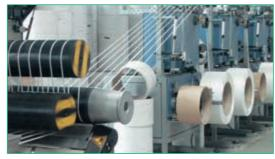
Fia. 4 Stretching process of Secugrid® ribs
