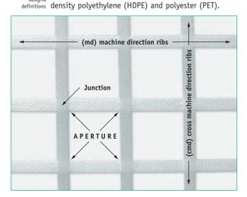
Geogrids are manufactured as either biaxial or uniaxial. Biaxial geogrids are those that exhibit the same strength in both the machine and cross machine directions while uniaxial geogrids exhibit the primary strength in the machine direction with minimal strength, enough to maintain the aperture structure, in the cross machine direction.
