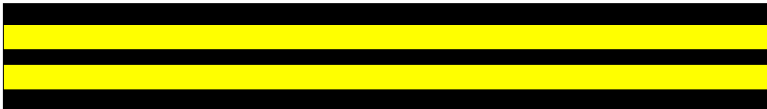
Continuous taxiway edge stripe
