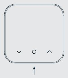
Remove the backplate of the thermostat by pressing the lever at the bottom and pulling away from the front of the device.
