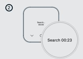
The thermostat display will show 'Search' – meaning it's searching for the Hub and Receiver. A timer will show how long the thermostat has been searching. If this lasts longer than five minutes, move the thermostat closer to the Receiver. Ensure the Hub is flashing amber; if not, press the button on the Hub briefly to start device pairing.
