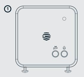
Loosen the screws on the underside of the Receiver and remove the backplate by pulling the bottom of it away from the front panel.
