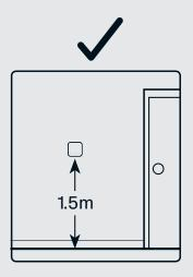
5b Wall mounting the thermostat
