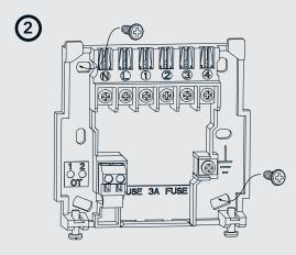
Fix the backplate to the wall with the terminals at the top.
