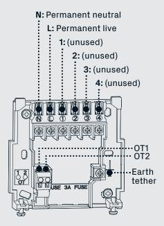
NOTE: If installing in OpenTherm mode, ensure you use separate cables for the low/high voltage connections. These should not share the same shrouding.
