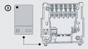
Run cable from the boiler or wiring centre (if required), then continue to the next section to wire up the backplate.
