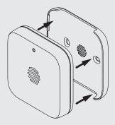
If using the included Hive Wall Mount, make sure appropriate wall fixings are used (the Wall Mount is designed for 3.5mm/size 6 or size 8 screws) and that the location is within suitable distance for the Bridge's power and data cables. Be careful to avoid any cables and pipes that may be buried in the wall.
