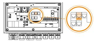
**Tip!** To connect the Hive Bridge to the Inverter you will need a suitably shielded Cat-5 (Ethernet) cable. If installing to an inverter with a combined canbus/RS485 port a suitable splitter will be required to complete the install.
