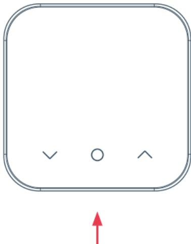
Remove the backplate of the thermostat by pressing the lever at the bottom and pulling away from the front of the device.
