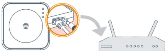
Connect the hub to the household's broadband router using the network cable provided.
