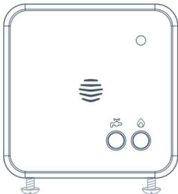
Loosen the screws on the underside of the receiver and remove the backplate by pulling the bottom of it away from the front panel.
