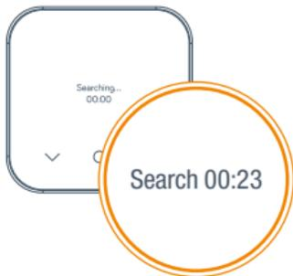
The thermostat display will show 'Search' – meaning it's searching for the hub and receiver. A timer will show how long the thermostat has been searching. If this lasts for longer than five minutes contact Hive Technical Support and they will diagnose any problems.
