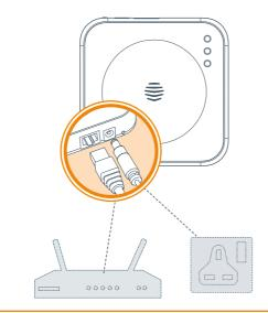
**Remember:** For your Hive devices to work correctly your hub must be kept plugged in and switched on.
