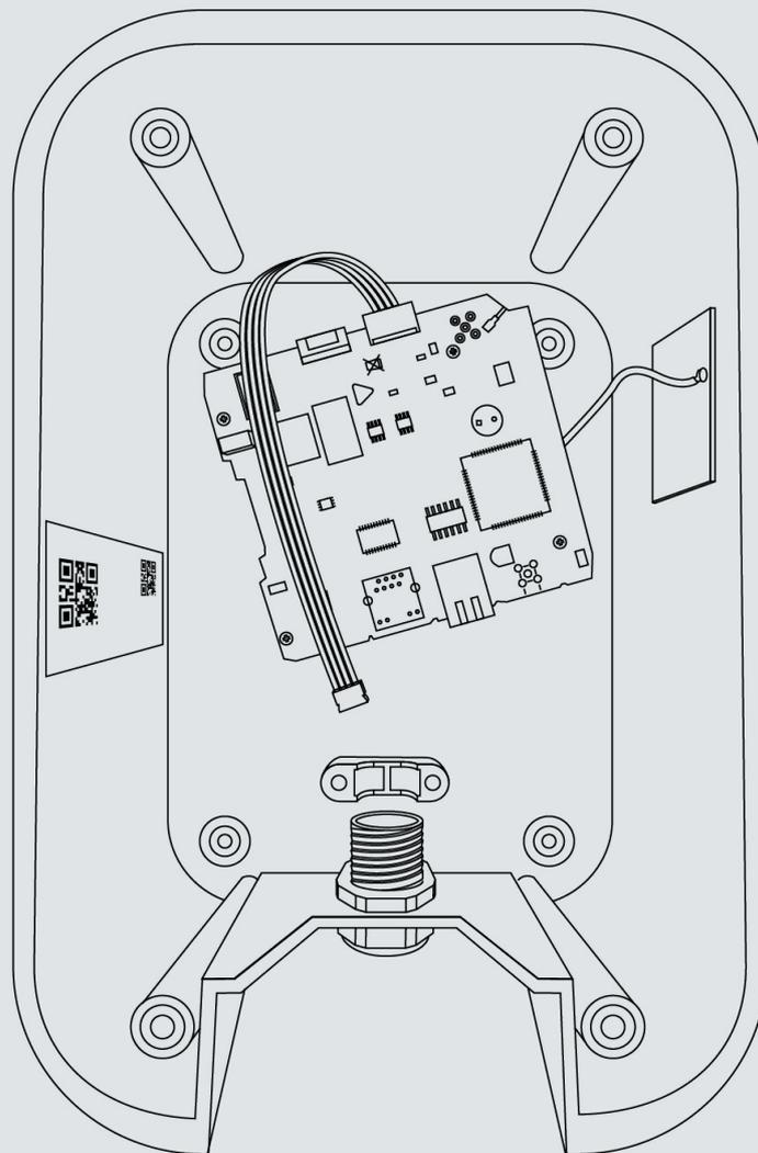
5. Attach the EO Mini Pro 3 base to the wall using the four screws provided. Make sure the charger is secure and flush against the wall. Use packing washers if necessary for a flush fit.
