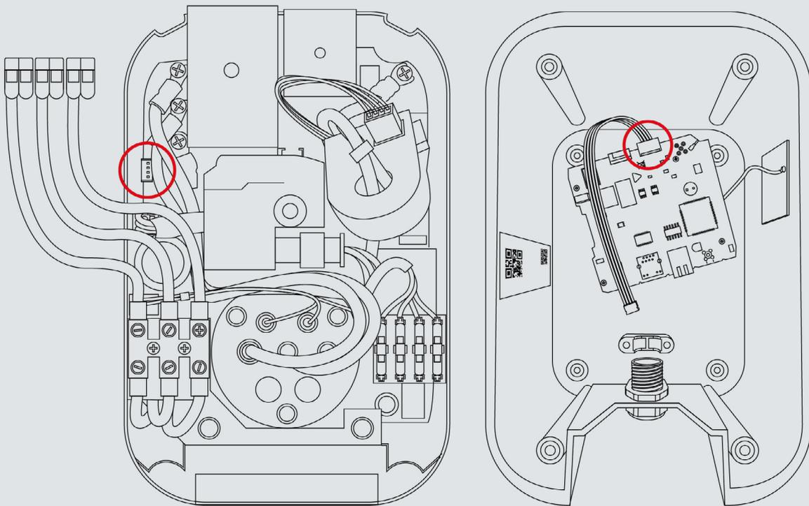
10. With all cables securely connected, close the Mini Pro 3 cases together, making sure no internal cabling is trapped, and secure the housings together with the four hex bolts and washers.
