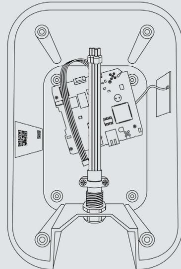
7. Connect the live, neutral, and earth wires to the charger connector block.
