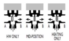
heating only position closing off the Hot Water circuit, the pump and boiler operate and circulate primary water to the heating circuit only.
