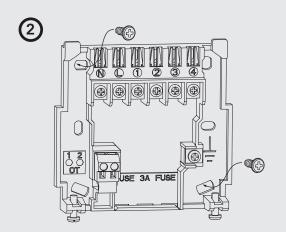
Fix the backplate to the wall with the terminals at the top.
