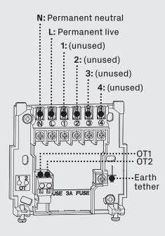
NOTE: If installing in OpenTherm mode, ensure you use separate cables for the low/high voltage connections. These should not share the same shrouding.
