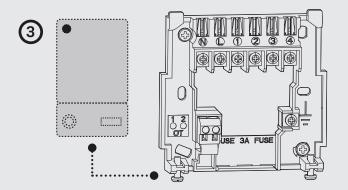
Run cable from the boiler or wiring centre (if required), then continue to the next section to wire up the backplate.
