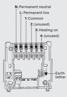
NOTE: Remove any existing controls or programmers and ensure pre-existing wires or connections are made safe.
