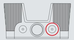
6. The rear charger housing allows for one rear cable entry using the position as shown on the image.
