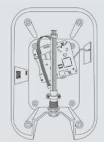
10. Connect the live, neutral, and earth wires to the charger connector block.
