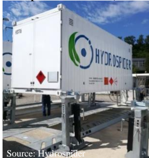
Compressor and Storage (500 & 1000 bar)
