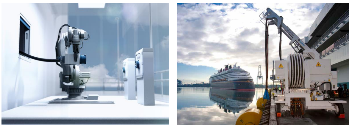
Figure 7-7: Automatic shore connection for charging electric vessels (left, Source: ABB) and telescopic crane for shore power connection (right, Source: Cavotec)
