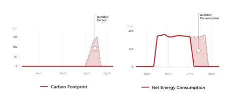
The IceBrick® allows you to store clean energy by charging when it's available—either from renewables onsite or from the grid—and when grid or price signals indicate it's cheap. Then, when the grid price is up, or renewable energy is out, the system can discharge the stored cold energy to generate grid revenue and maintain uninterrupted cooling without resorting to carbon-intensive, costly afternoon-evening grid electricity.
