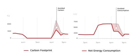
The IceBrick® allows you to store clean energy by charging when it's available—either from renewables onsite or from the grid—and when grid or price signals indicate it's cheap. Then, when the grid price is up, or renewable energy is out, the system can discharge the stored cold energy to generate grid revenue and maintain uninterrupted cooling without resorting to carbon-intensive, costly afternoon-evening grid electricity.
