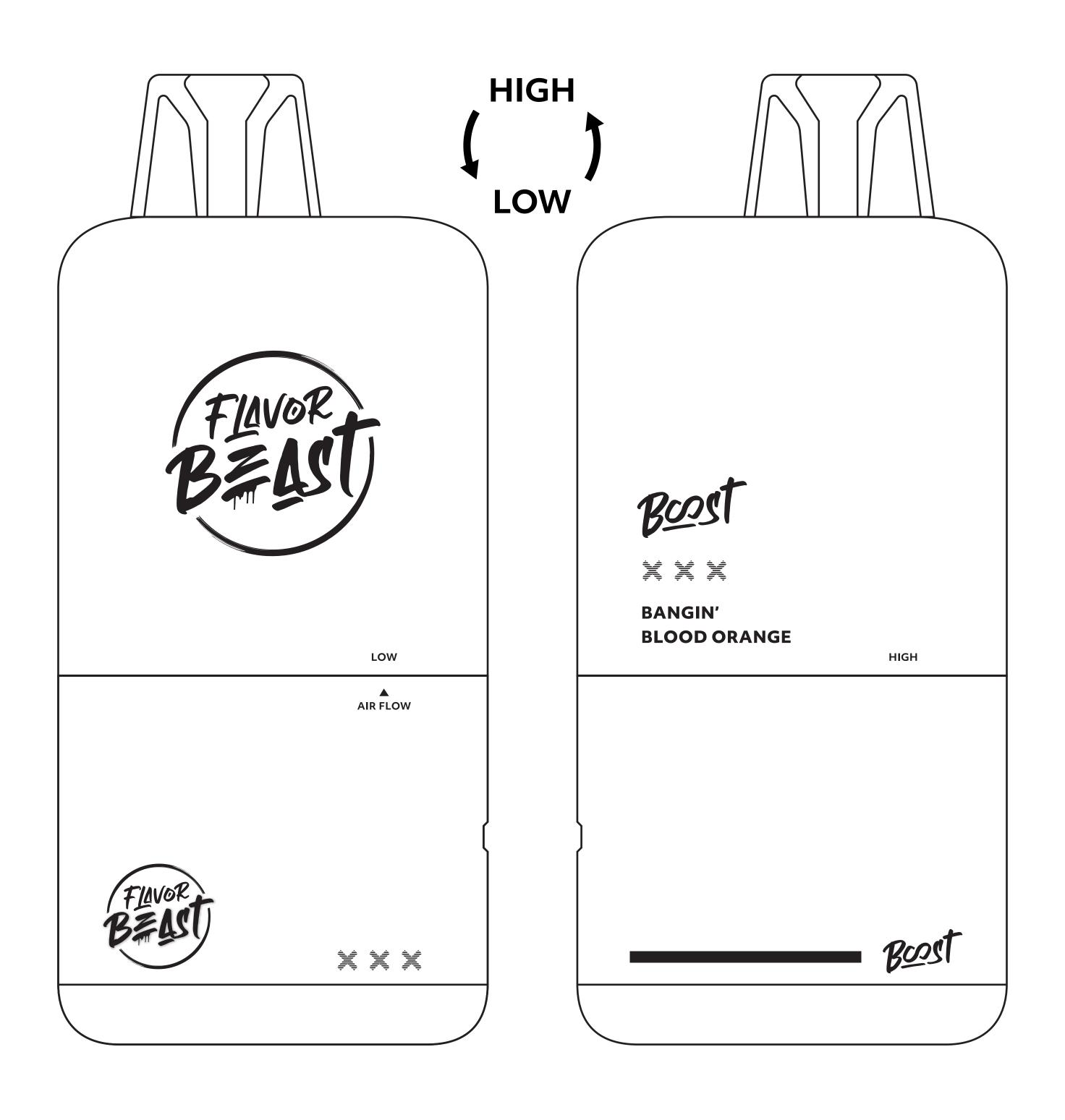
2. Attaching the pod in either of the two orientations will result in different airflow options.
