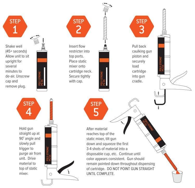
**Note:** Cartridge should be stored or conditioned to 65°F - 75°F prior to use.
