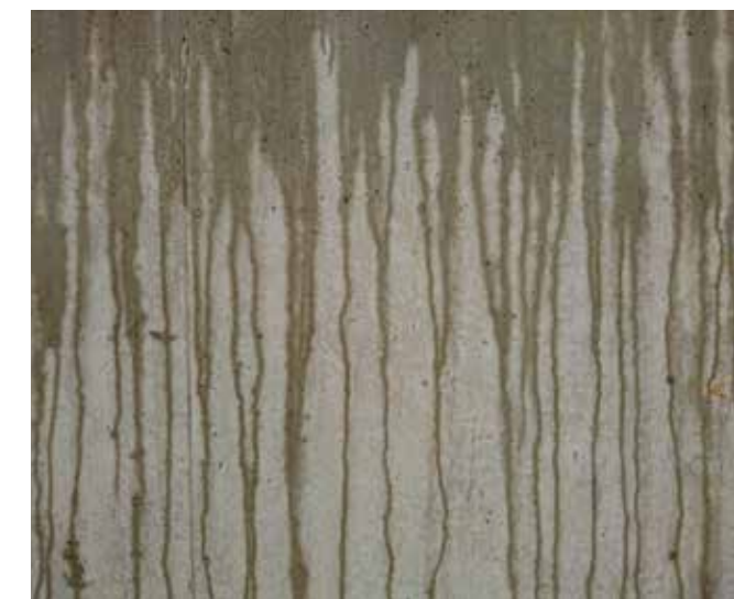
Traditional silanes on vertical surfaces are prone to excessive run-off. Excessive run-off leads to low penetration, significant material loss and poor performance.
