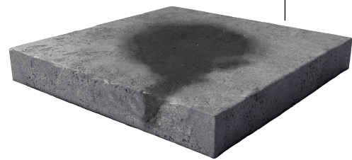
Untreated Concrete, Showing Chloride Intrusion
