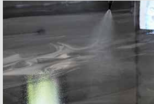
SPRAY USING A CONE TIP FINEST MIST WILL ACHIEVE THE BEST RESULT
