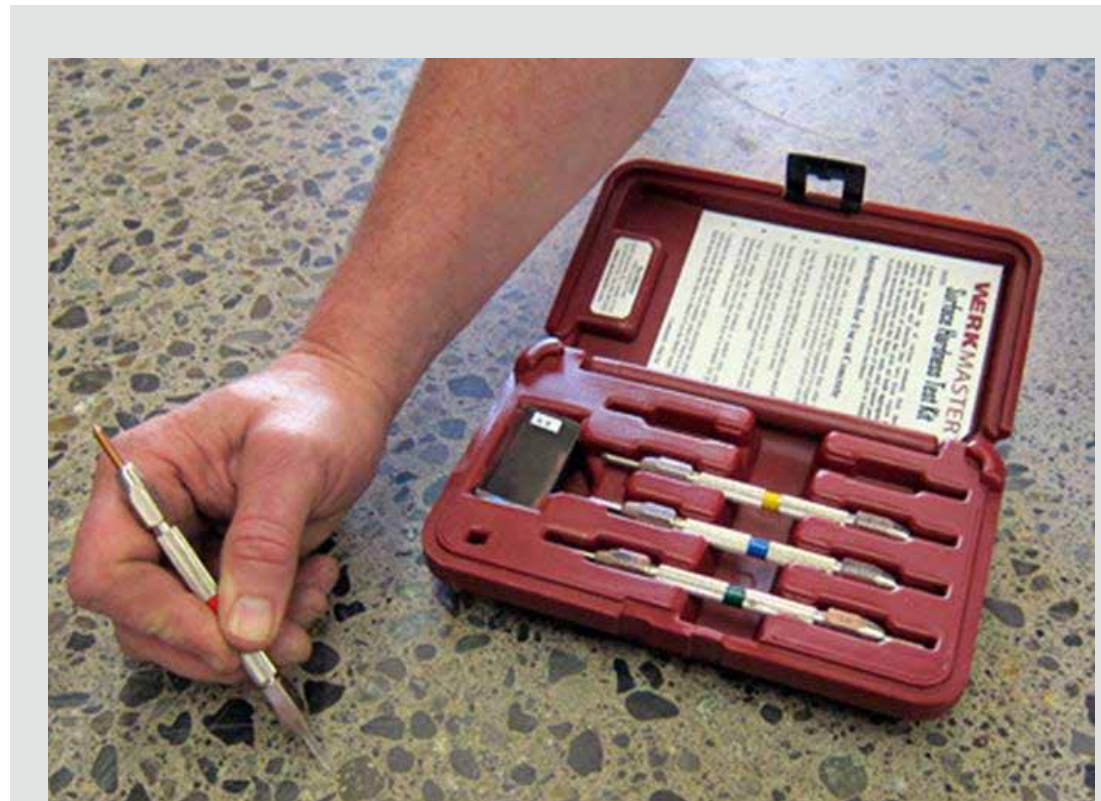
MOH HARDNESS TEST KIT STANDARD MINERALS TO MEASURE SCRATCH RESISTANCE
