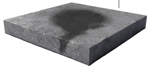
Untreated Concrete, Showing Chloride Intrusion
