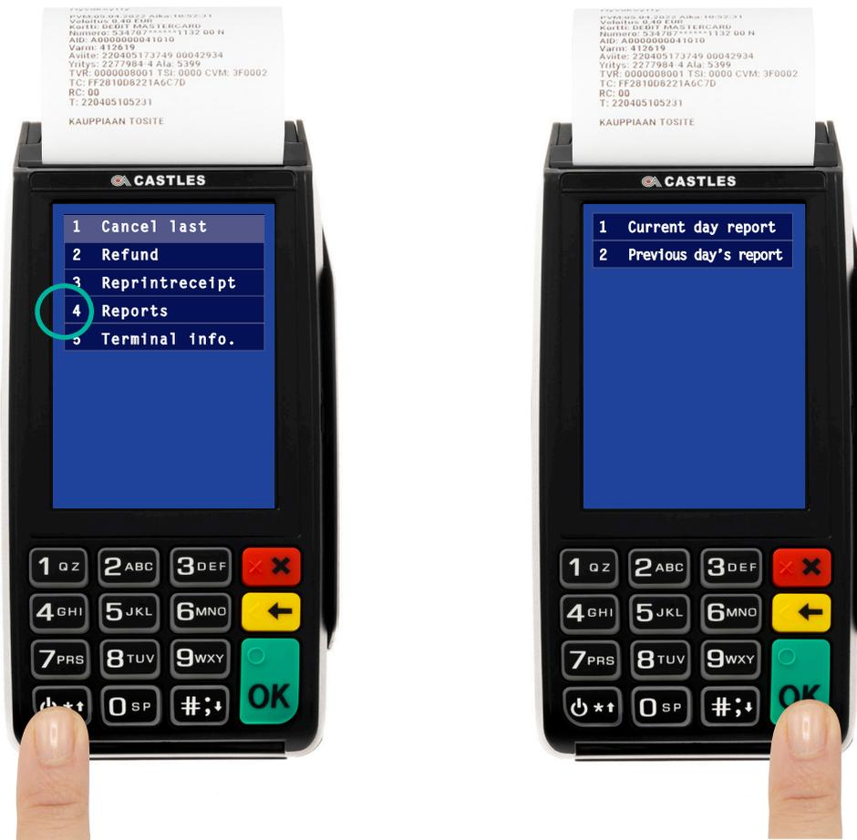
Press the **power/menu key** in the left corner of the terminal for displaying the menu on the terminal screen.
