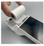
2. Insert the paper roll in the compartment following the directions shown in the picture.
