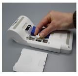
2. Insert the battery plug into the socket and insert the battery into the battery compartment.
