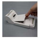
1. Turn the terminal upside down and open the battery cover.
