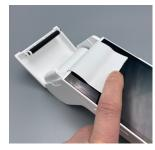
3. Pull 5 cm of the paper until it protrudes from the compartment on the top of the terminal.
