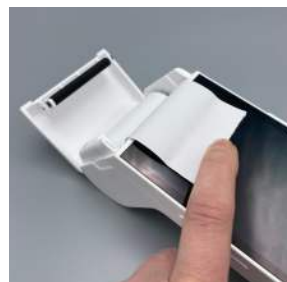
3. Pull 5 cm of the paper until it protrudes from the compartment on the top of the terminal.
