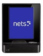
This terminal hardware is designed for self-service environments namely Unattended use cases such as EV-charging, and only provides contactless interface, means cards can not be inserted in the payment terminal. Terminal doesn't have any physical keys, which means that the onscreen navigation is done directly from the displays own capacitive touch screen.
