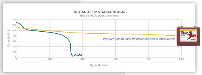
Trojan AES maintains high capacity in extreme deep-cycling (up to 100% DoD) with consistent performance throughout its life compared to standard AGM.
