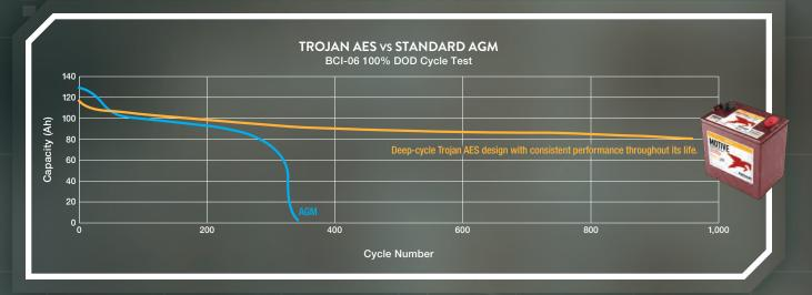
The "AES" in "Trojan AES AGM" stands for "advanced energy storage" and is Trojan's latest deep-cycle battery breakthrough, offering up to 3X the cycle life of standard AGM, great performance in extreme temperatures, and withstanding PSoC again and again. We gave AGM batteries a facelift to give you longer-lasting batteries.
