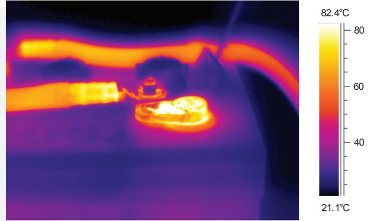
It is therefore highly recommended that connectors not only be mechanically crimped but also soldered to the cable's end. A properly crimped and soldered connector will provide a low resistance connection and reduce the amount of heat buildup at the connecting junction.
