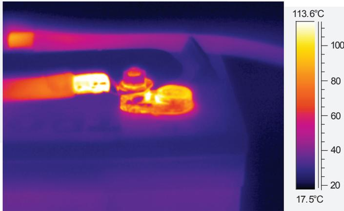
The infrared picture below shows a cable with crimped and soldered connector under a high-rate discharge. Note that the high temperature area is no longer near the connecting junction but evenly distributed along the cable and battery terminal.
