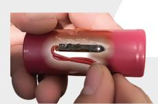
Internal temperature sensors are a key component in lithium-ion battery charging and safety. They provide critical temperature data required to keep the lithium-ion battery in the optimum condition during the charging cycle.
