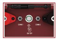
**Power On/Off:** Locate the ON/OFF Power Switch on the side of the battery in-between the power terminals.
