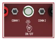
**Turning Off:** Press the button, hold for approximately 6 seconds, and release. Verify that the green LED is no longer blinking.
