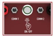
**Turning Off:** Press the button, hold for 6 seconds, and release. Verify that the green LED is no longer blinking.
