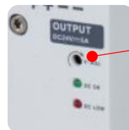
DC Output Potentiometer
