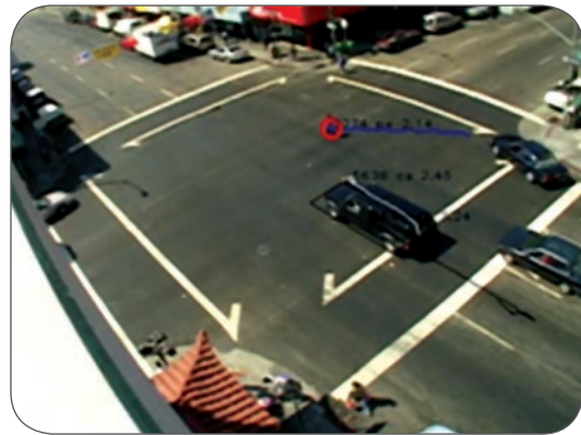
Figure 2: A sample of automatically detected pedestrian-vehicle conflict in a before and after safety study of a pedestrian scramble phase in California (Source: Ismail, Sayed and Saunier, 2010)
