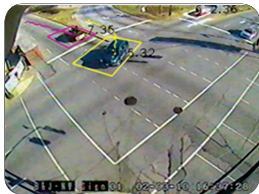
Figure 3: A sample of an automatically detected vehicle crash in a safety study in USA (Source: Saunier, Sayed and Ismail, 2010)
