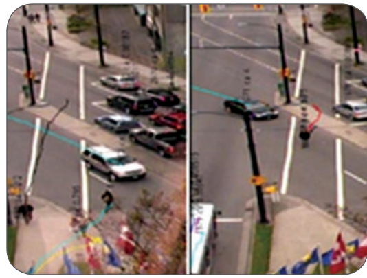
Figure 1: Sample of automatically detected pedestrian-vehicle conflicts in a Downtown Vancouver study (Source: Ismail, Sayed and Saunier, 2009)
