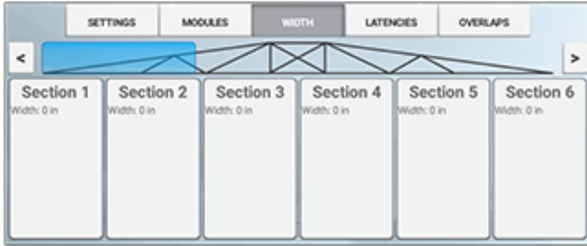
This screen will show the measured section width for each section on the boom. The widths of individual sections can be changed by pressing on the section button. Note that total boom width cannot be changed from here. Any changes made to individual sections will result in the altering of the width of the **last** section in order to maintain a constant boom width.
