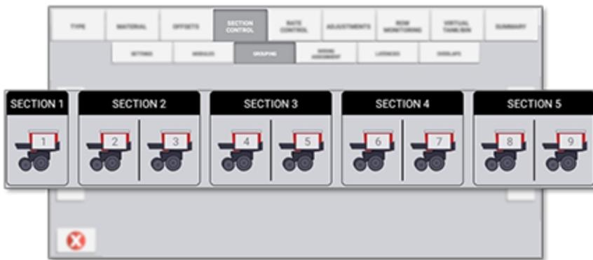
**NOTE** - Sections are modified by adding new rows to sections (A row can't be removed from a section, only added to another). For example, if Section 1 contains rows 1 and 2, to move row 2 to section 2 the user would tap on section 2 and add that row to the section.
