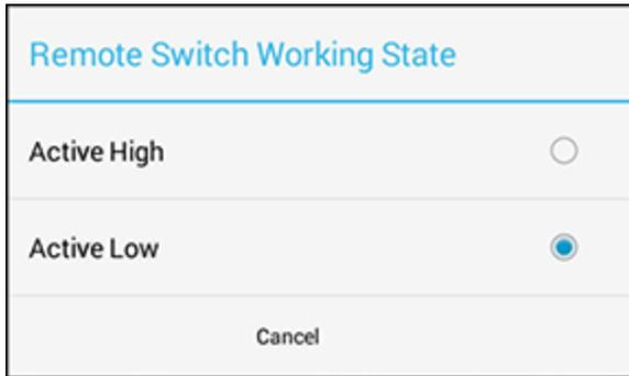
**Active High:** the circuit is open (The display is sensing that the reference signal voltage is not completing a circuit).
