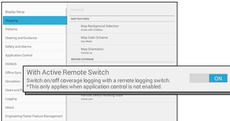
**NOTE** – If you use the **With Active Remote Switch** option, then the **When Engaged** option cannot be enabled
