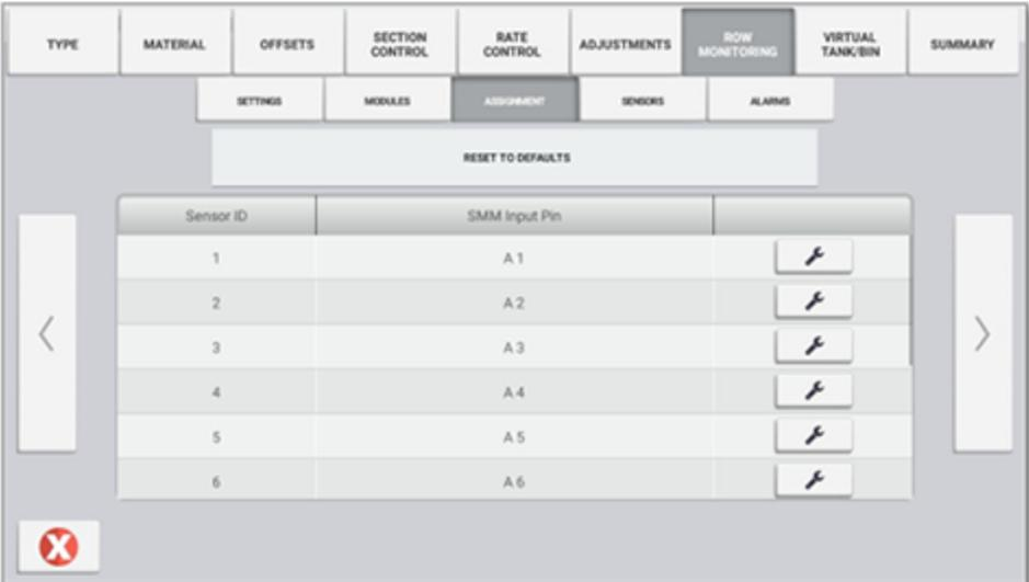
To modify an input, tap the wrench icon next to that input. A list will show indicating the inputs current sensor assignment. To change the assignment, select the new input (inputs that are already assigned will be overwritten).
