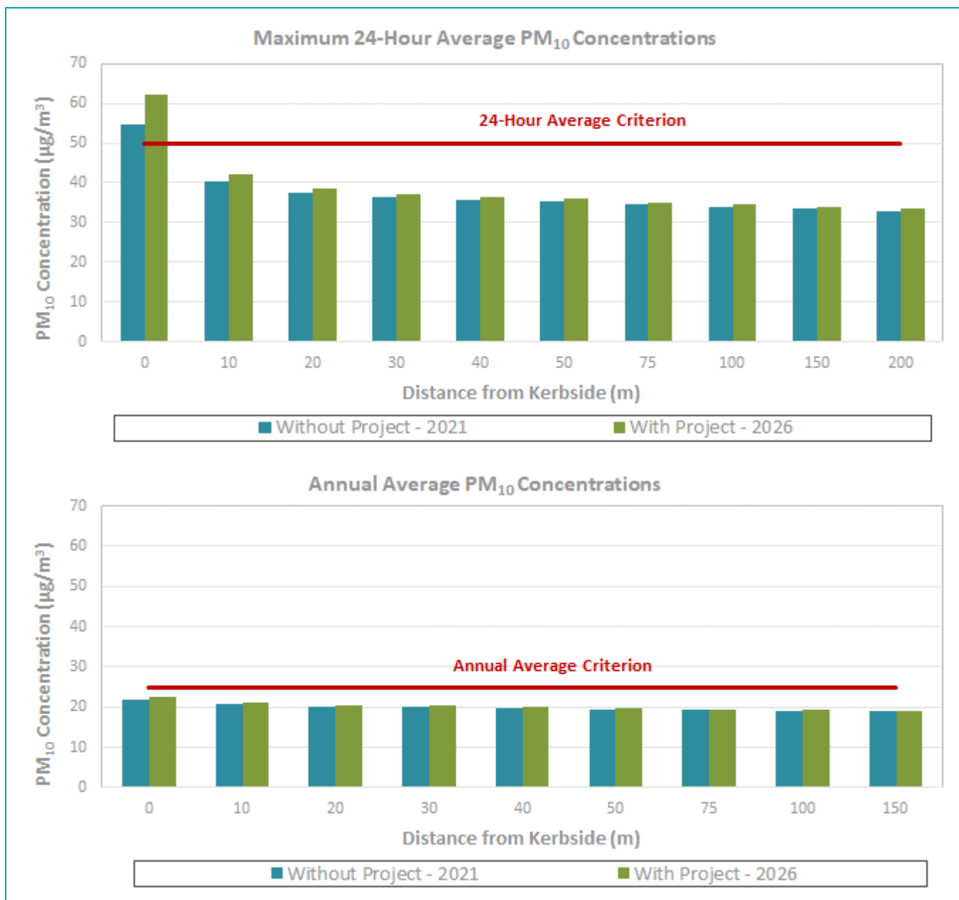
Figure 16 Maximum Predicted PM 10 Concentrations Versus Distance from Mamre Road and Abbotts Road (TRAQ)
