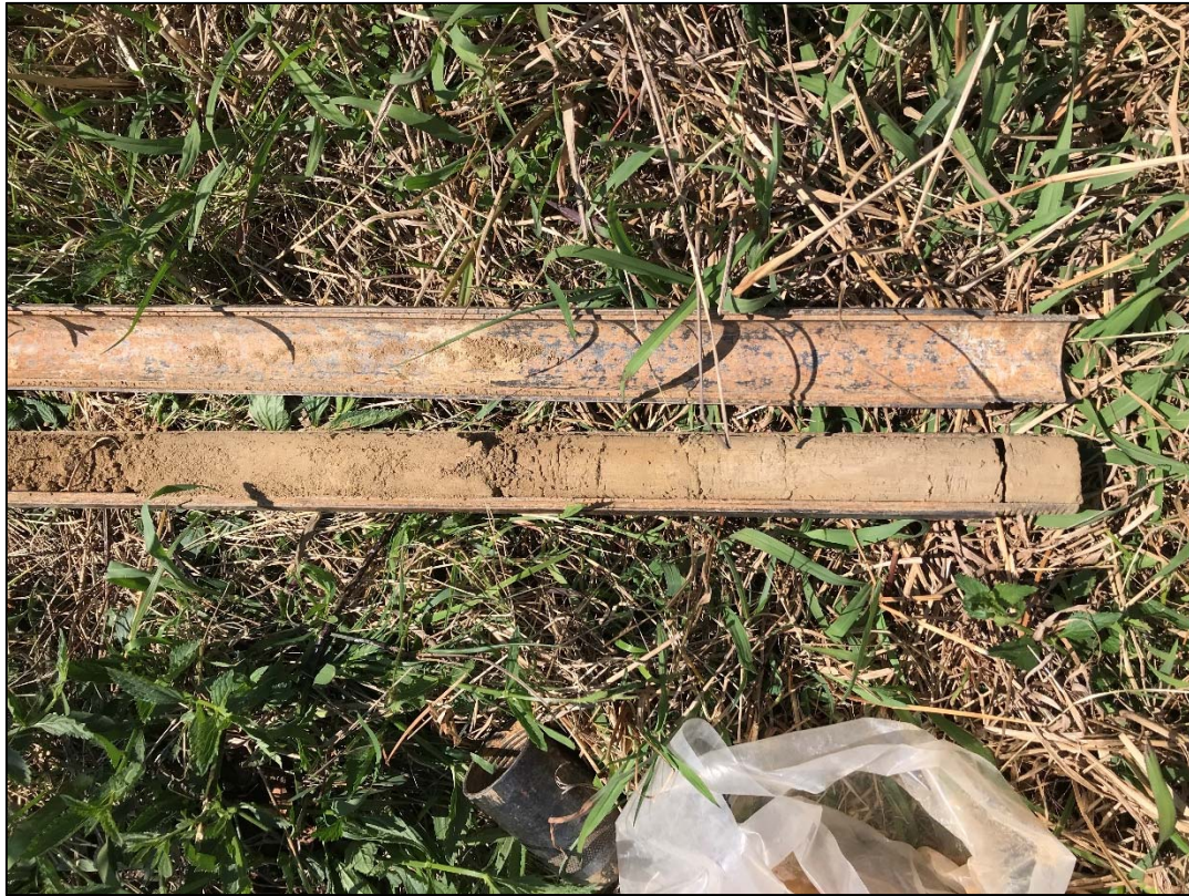
Figure 3 – SPT sample retrieved from residual soil after the test
