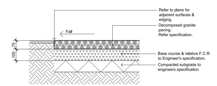
04 DG - Decomposed Granite Paving on Grade
