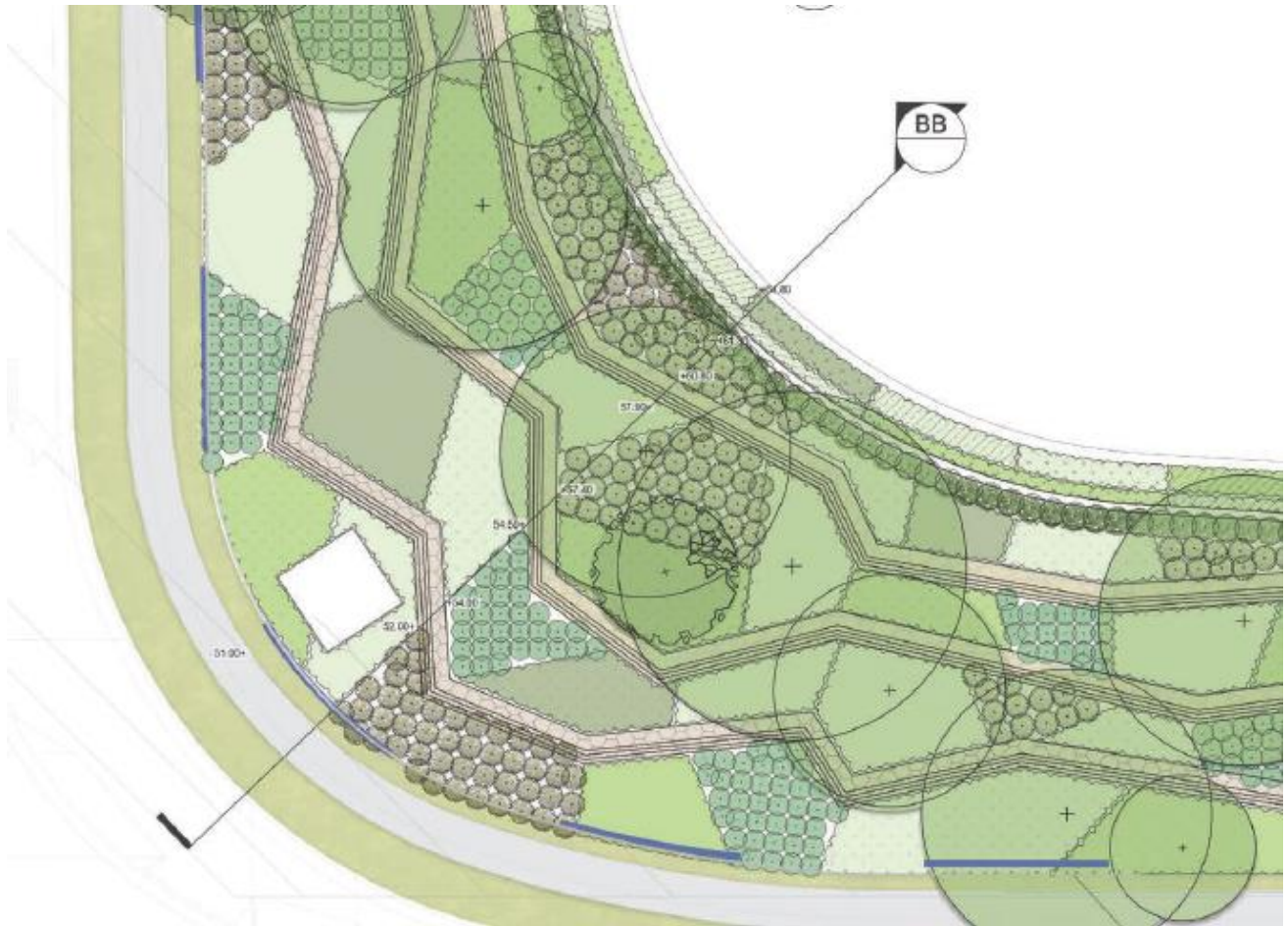
Figure 4 Plan view of Aldington Road retaining wall showing the zig-zag and larger canopy trees
