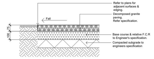
Decomposed Granite Paving on Grade
