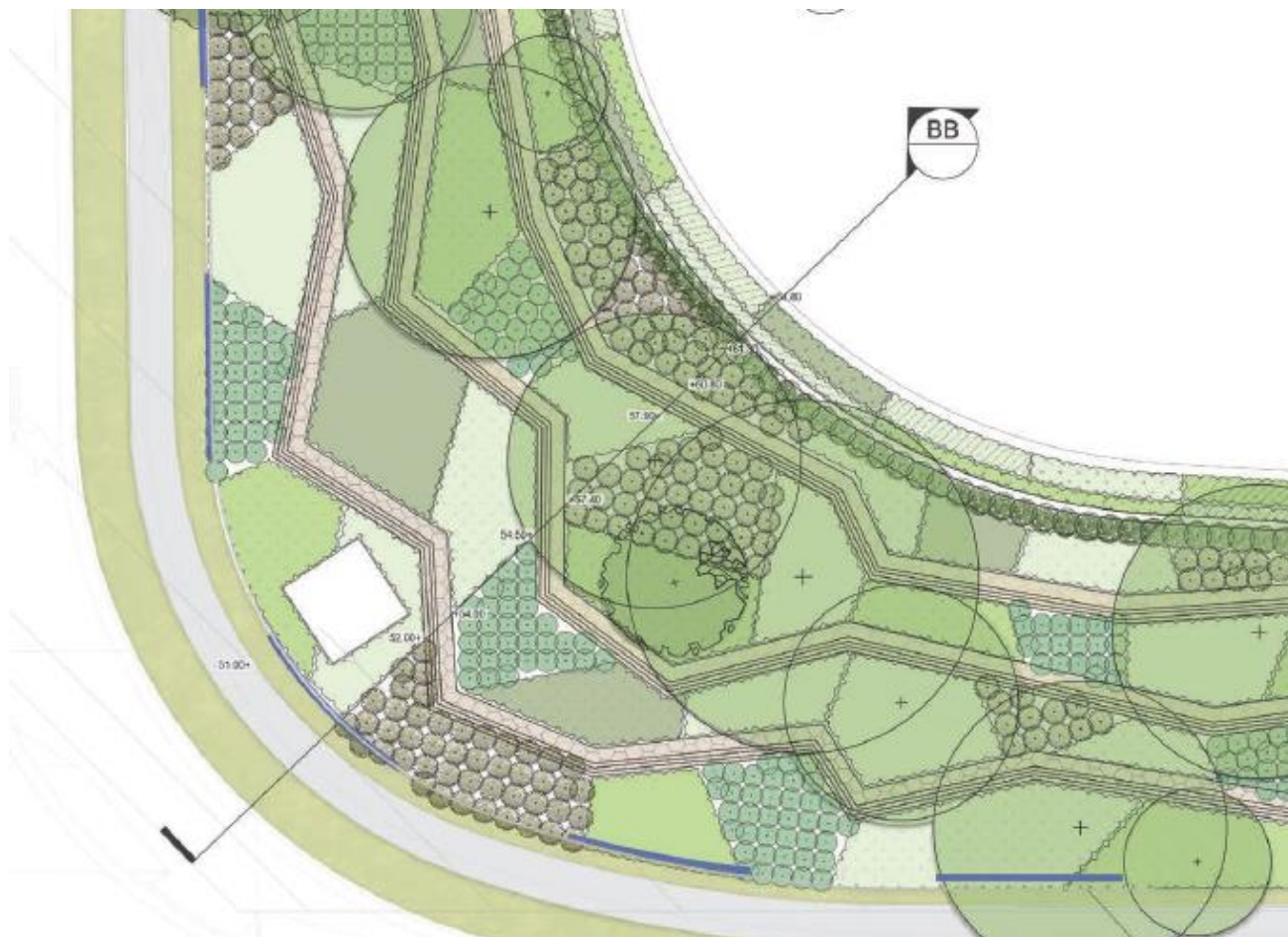
Figure 4 Plan view of Aldington Road retaining wall showing the zig-zag and larger canopy trees
