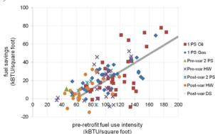
Figure 18: Capped Projected Fuel Savings vs. Pre-Retrofit Fuel Use Intensity
