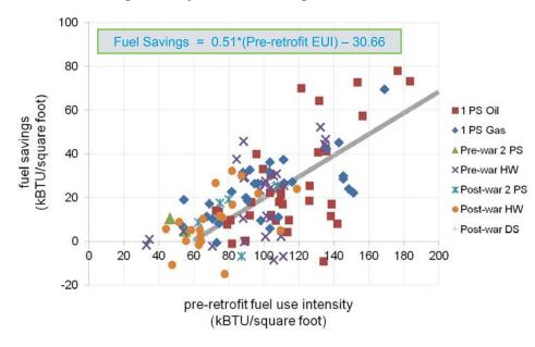
Using regression analysis, the team derived an empirical model that identified the linear relationship between a building's post-retrofit savings and pre-retrofit fuel consumption. This relationship, depicted by the grey line in the chart above, represents the only statistically significant trend identified in post-retrofit performance relative to pre-retrofit characteristics in the DB/LC dataset.
