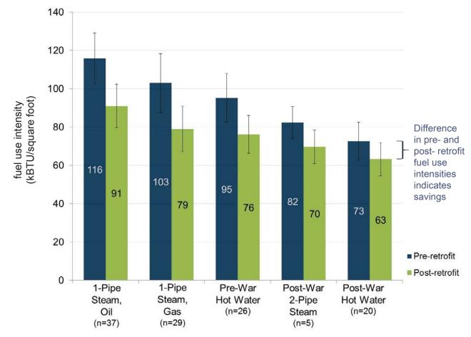
The error bars shown on the chart represent half standard deviations above and below the mean for each comparative group. If multifamily buildings were normally distributed along a bell curve, the range would approximately represent the middle 40%.
